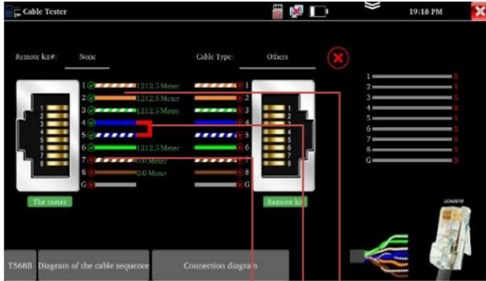
Test cable's continuity, length and fault locator of RJ45 cable connector. The number of the cable tester is 255.
