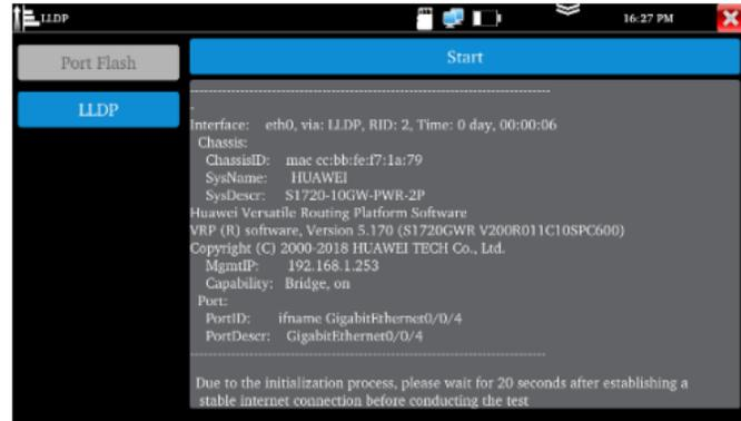
Used to detect the main capabilities, management addresses, device identification, interface identification, and other information of switches and other devices.
