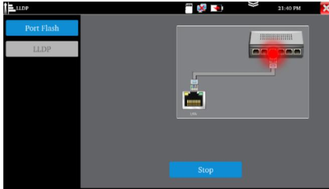
Quickly find the connected Ethernet cable
