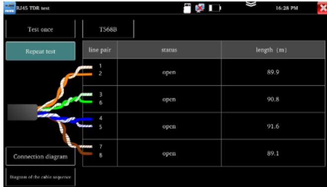
Connect cable to the LAN port of tester, the other end connects or disconnect other device. Enter “RJ45 cable TDR test” app to test cable’s length. Test cable’s length, please don’t connect any device. **The max measurement length is 600 meters.**
