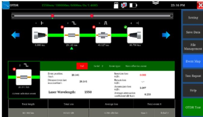
Display the quantity of event, link loss, link length, link attenuation coefficient. Click again to switch to trace.
