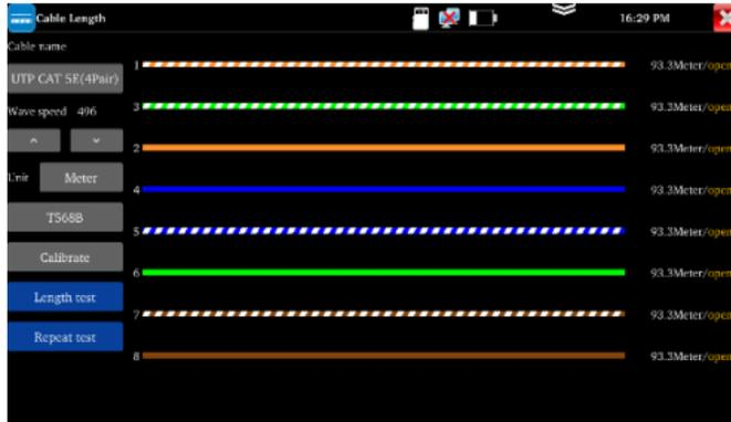
Note: The measured cable cannot be connected to any device. If connected to other devices, it will cause incorrect measurement results!
