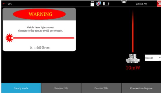
It is used to determine the continuity of optical fibers and locate faults
