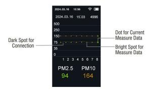
In the measurement page a LONG PRESS of the MEM/Down button enters and exits the memory page.
