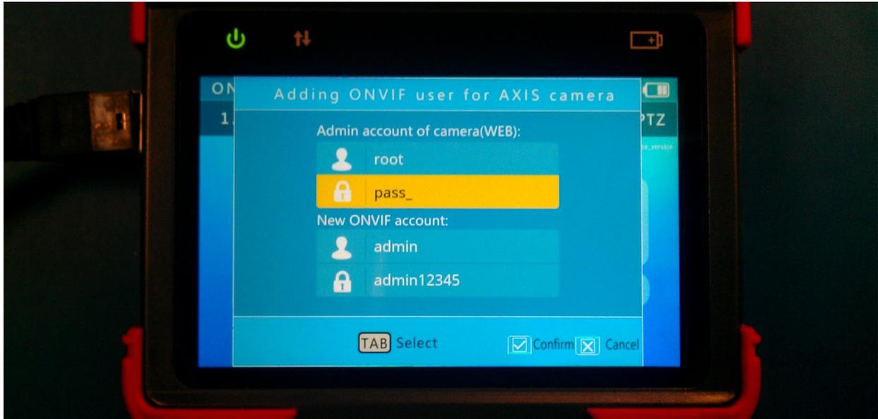
If the new user is successfully created, the tester will return to the “Discover” screen and automatically log in to the new ONVIF user. At this point, the user can press the “SET” button to enter the camera settings, where additional usernames can be created (or deleted) with different levels of access. Once logged in to the ONVIF user, press the right arrow button to view the video stream.
