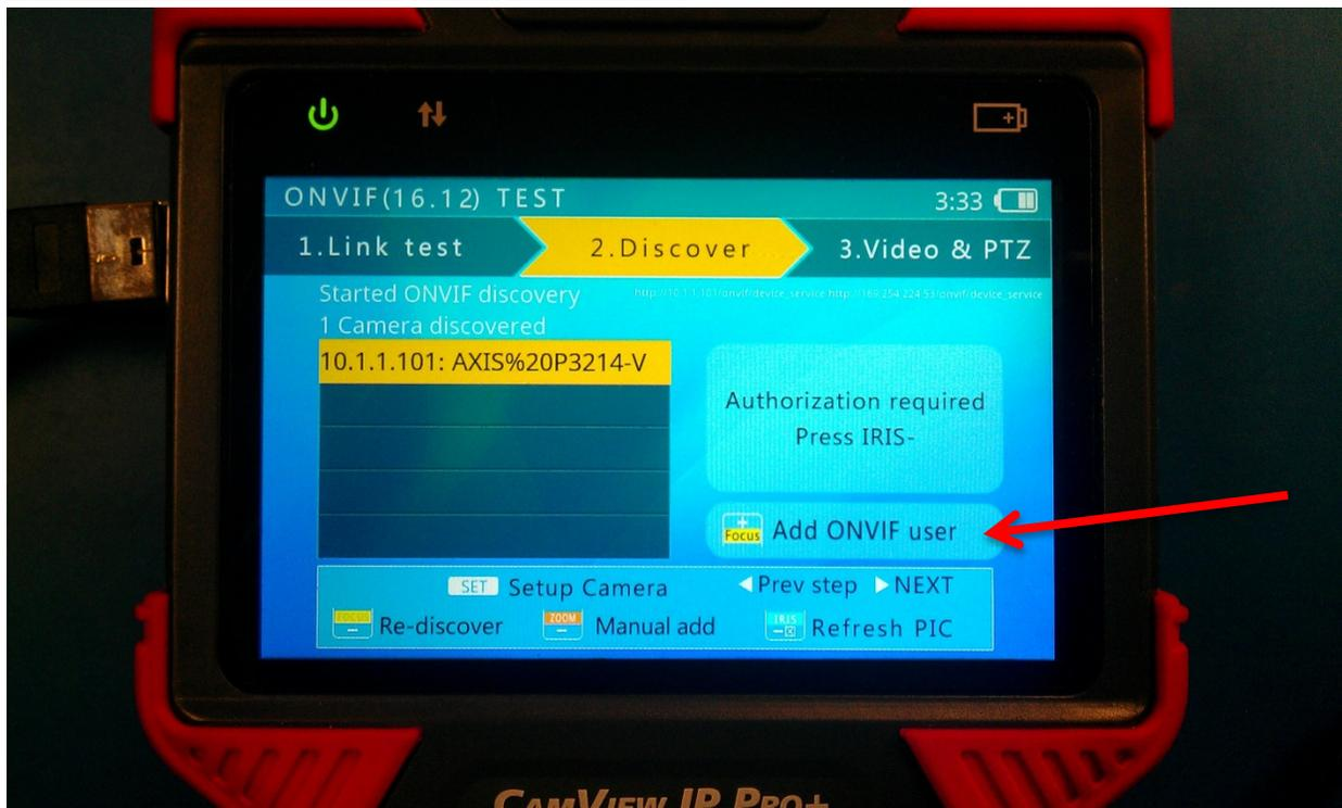
In the “Add ONVIF user” screen, the tester defaults to the following entries. Use the “TAB” button in the swing out keyboard to switch entry fields. Change the usernames and passwords as necessary. The default username for Axis cameras is “root”, with the password “pass”.
