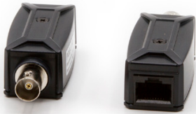
POE-1TR IP Extender over Coax Pair Does not support PoE
