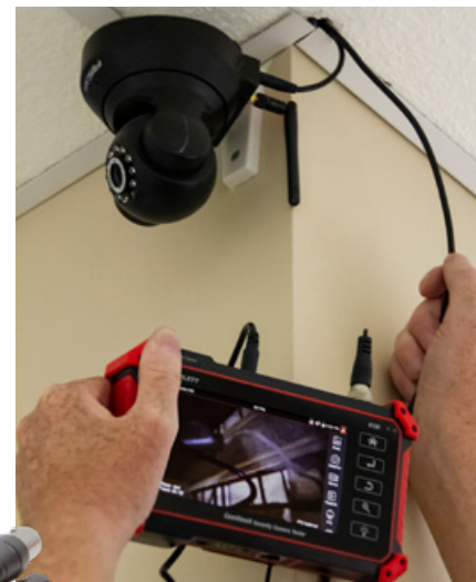
SBR2M borescope with Triplitt model 8150 CamView5 Security Camera Tester
